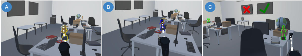
Figure 1: 3DUI authentication virtual environment with HOG interaction technique used in this paper: (A) Selectable authentication token highlighted. (B) Authentication token highlight on selection. (C) Updated virtual environment on successful authentication with verified token highlights.
