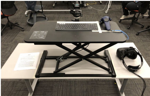
Figure 2: Physical apparatus with Logitech Wireless K780 keyboard, HTC Vive Controller, HTC Vive Tracker, and Varjo XR-3 HWD.
